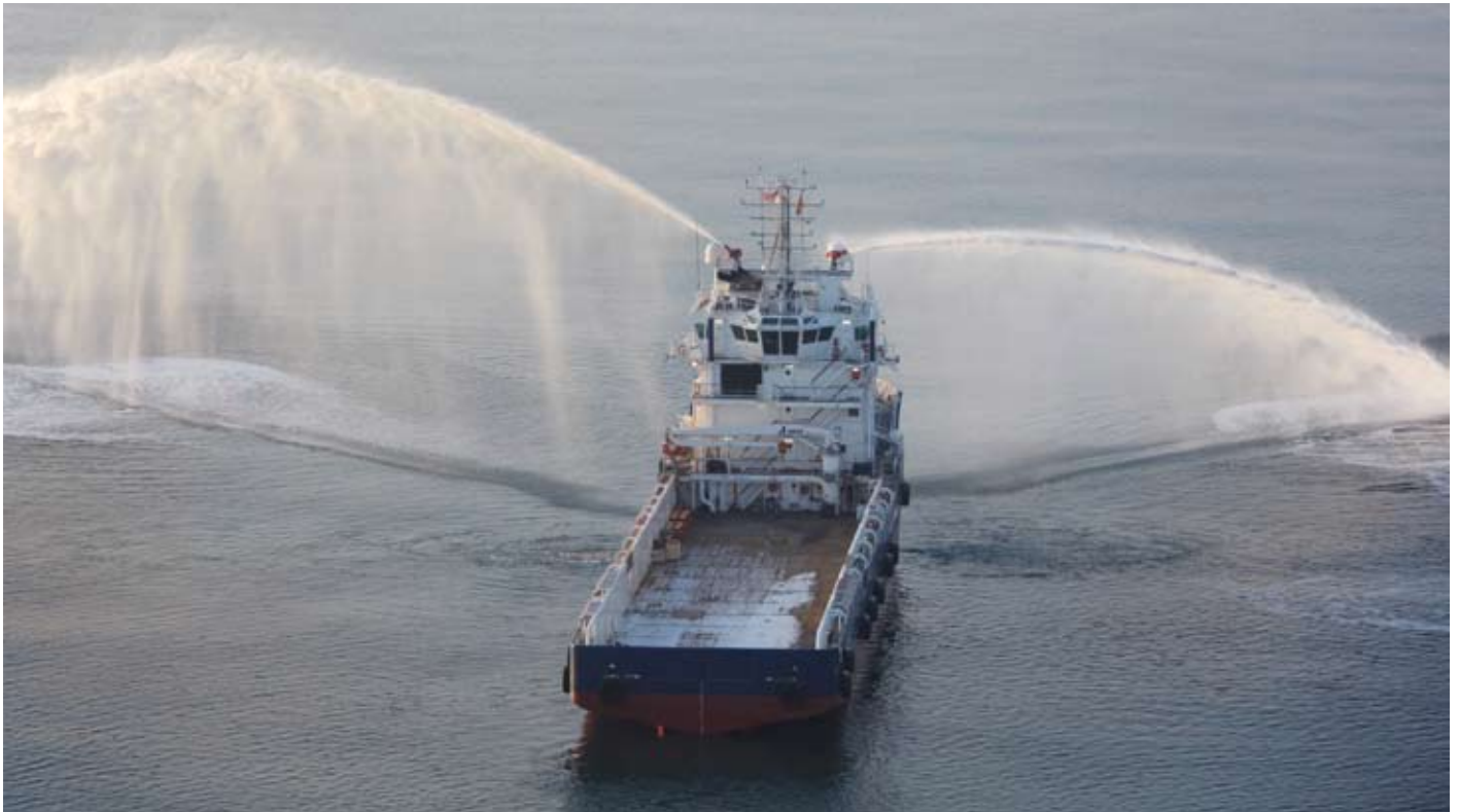
Platform Supply Vessel GO COUGAR, of a Rolls Royce UT 755 LN design, built by Aker Aukra Norway after upgrading the DP2 positioning system on sea trials in the North Sea.
