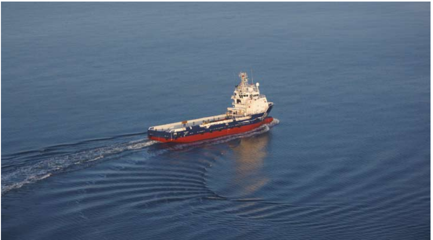
Platform Supply Vessel GO COUGAR, of a Rolls Royce UT 755 LN design, built by Aker Aukra Norway after upgrading the DP2 positioning system on sea trials in the North Sea.
